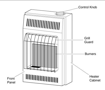
Figure 1 - Vent-Free Propane Gas Heater (Model VP11 Shown)
